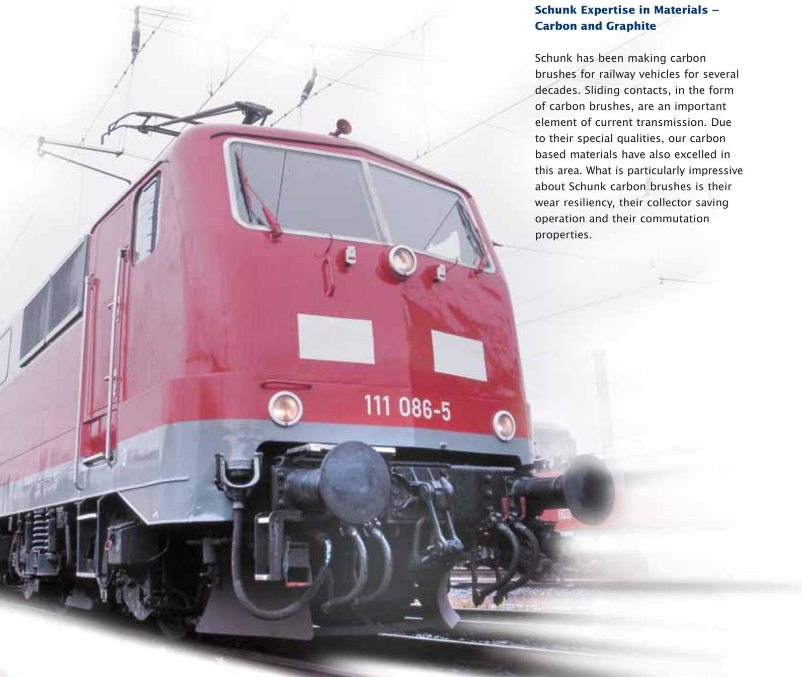
*One of the most proven locomotives of the German Rail service (BR111). With collector strips, traction-motor carbon brushes, brush holders and grounding contacts from Schunk*
