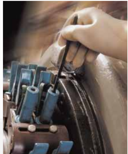
Inspection of the carbon brush with the motor running, using the Schunk Measuring stick (can be acquired from Schunk).
