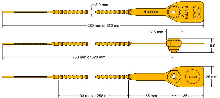
The Acme **Griptight Seal** is a heavy duty pull-tight seal manufactured from two dissimilar materials. The acetyl insert is durable and will withstand freezing and boiling conditions, whilst the nylon body is flexible for easy use. The design features rolled heat staking technology to secure the insert to the body, which provides clear evidence of tampering if forced open or cut. This seal is suitable for most applications where strength is a requirement.
