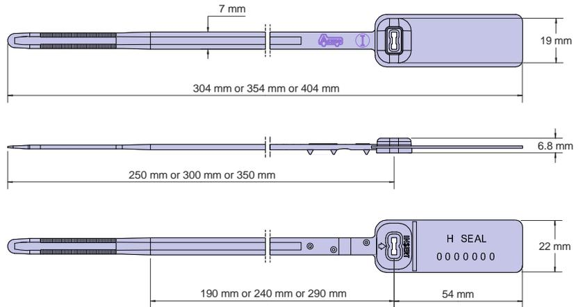
The Acme **H Seal** is a smooth ribbon, pull-tight seal manufactured from Polypropylene material. The design features rolled heat staking technology to secure the metal spring insert to the body, which provides clear evidence of tampering if forced open or cut. The seal can be manufactured with or without gripping spikes, making this seal suitable for many applications where strength is the requirement.
