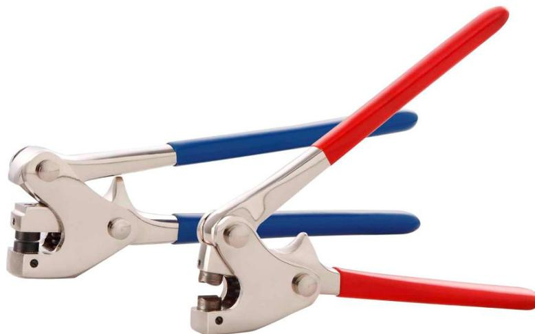
The Acme **Sealing Tools** are manufactured from cast carbon steel and chrome plated for protection. The tools are supplied with round dies, plain or corrugated for effective crimping of all Acme Lead Seals, the plastic YP10 and Crimp Seals. Non standard engraved dies can be supplied to emboss or deboss characters or numbers onto the seal when it is crimped closed. The sealing tools may also be used to mark other materials such as aluminum plate or laminated card.
