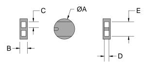
The **Round Lead Seal** is designed with two parallel holes and a knot chamber. During fitting the wire or string is threaded through the two parallel holes and crossed inside the knot chamber before closing with the sealing tool to prevent slippage.
