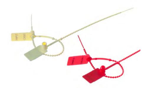
The Acme **F Seal** is a low breaking strength pull-tight seal manufactured from Polypropylene material. The seal can be supplied with a heat rolled over top to prevent tampering by intrusion into the locking head but if tampering is not the main characteristic the seal can be supplied without this added feature. With a 2.6mm diameter ribbon this seal is ideal for applications where there are small sealing apertures.
