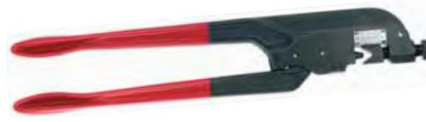
For preinsulated tubular lugs from 10 to 95 mm<sup>2</sup>
