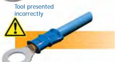
Cable over stripped, difficult to assemble on the tab
