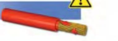
Cable insulation damaged
