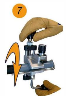
When you arrive at the stripping limit (end of the gratuated gauge in contact with the core), stop the tool Office Bitola:
