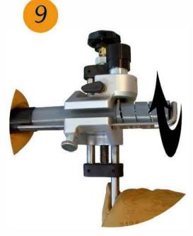
Finish with the straight cut turning 2 turns
