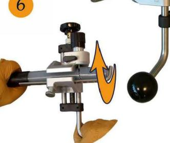
Introduce the gratuated gauge and lock at the needed position
