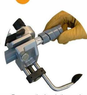
Remove the insulation and the tool
